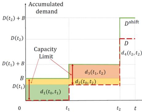
Fig. 1 Example for one-shot load decomposition
